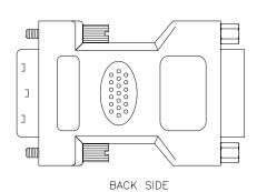
1.DVI (18+1)M:DVI—Digital 19P Male Connector Insulator: High Temperature Plastic UL—94V—0 Contact: Shell: Steel With Tin Plated 150u'' Over Contact Plating: Gold On Contact Area
